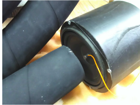
Fig. 4. The speaker and the accelerometer the signal is increased in steps covering the frequency band of interest roughly from 50Hz
