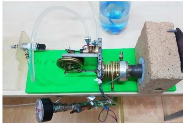
**Fig. 3.** Experimental installation for determining the flow of water through the cooling circuit (cooling variant 1).
