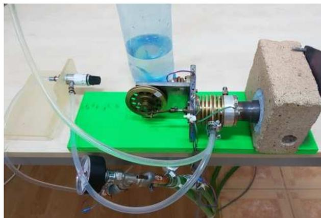
**Fig. 4.** Experimental installation for determining the flow of water through the cooling circuit (cooling variant 2).
