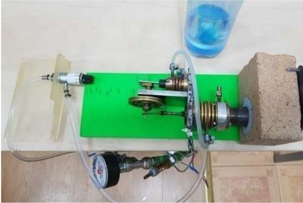
**Fig. 5.** Experimental installation for determining the flow of water through the cooling circuit (cooling variant 3).
