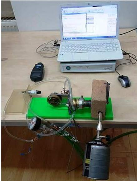
**Fig. 10.** Experimental installation for determining the speed in cooling version 3.
