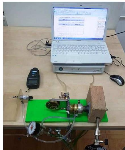
**Fig. 9.** Experimental installation for determining the speed in cooling version 2.
