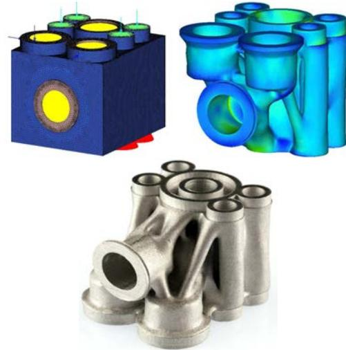
**Fig. 10.** Steps to Redesign and AM processed of a hydraulic valve block for heavy-duty [19]
