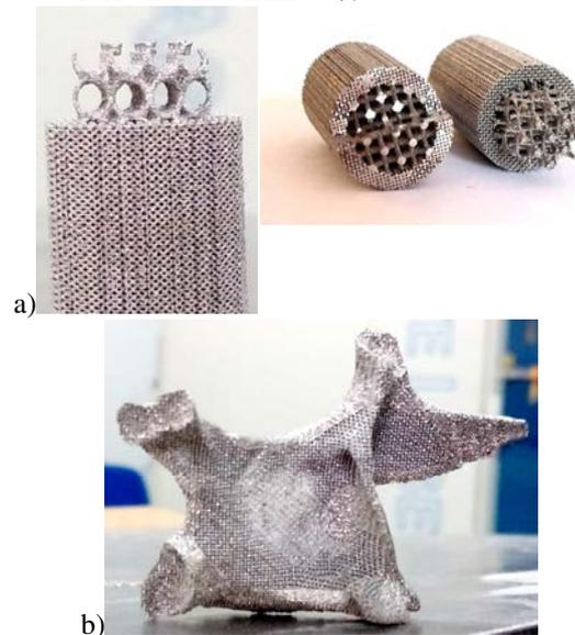
**Fig. 16.** Implants SLM-manufactured with lattice structures: a) Medical grafts with variable porosity, b) Maxillofacial reconstruction with solid outer boundary and macro-porous area [28]
