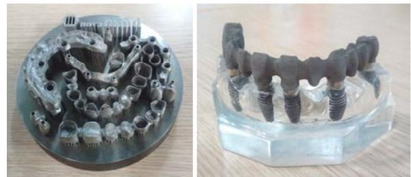
**Fig. 13.** Dental applications SLM-manufactured from CoCrWMo, [www.novamind.gr](http://www.novamind.gr)
