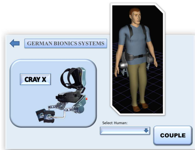
Fig. 7. Vision of a GUI for coupled exoskeleton (© Fraunhofer IAO).
