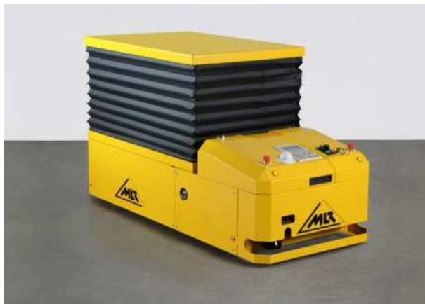
Fig. 9: example of an automated guided vehicle [19]
