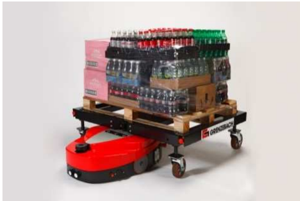
Fig. 8: example of an automated guided vehicle [18]
