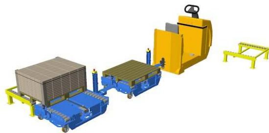
Fig. 6: automated loading of large load carriers [16]
