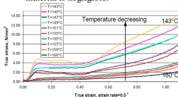
Fig 2: Isothermal stress-strain curves obtained by testing polypropylene (temperature range 143 ÷ 160°C, constant velocity) [5]
