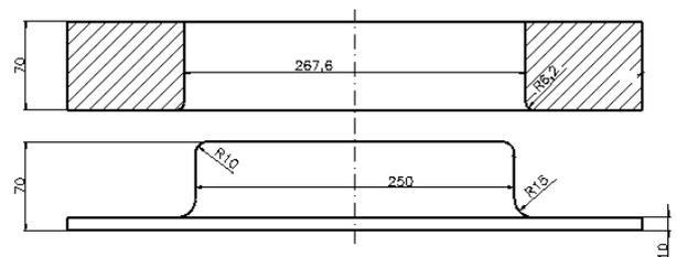
**Fig 3: Characteristics of the thermoforming mold**
