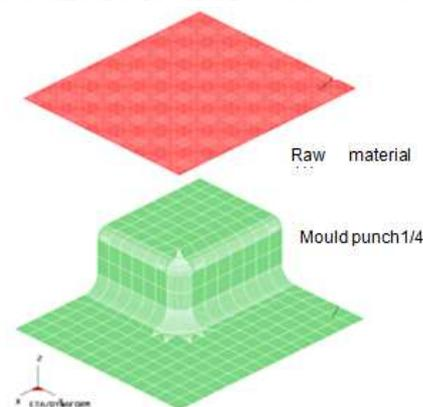
Fig 4: Finite element meshing of the components of the gravitational deformation process
