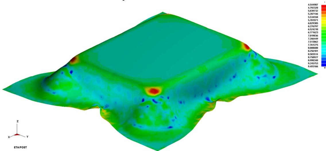
**Fig 5:** Thickness distribution at the end of the gravitational deformation process
