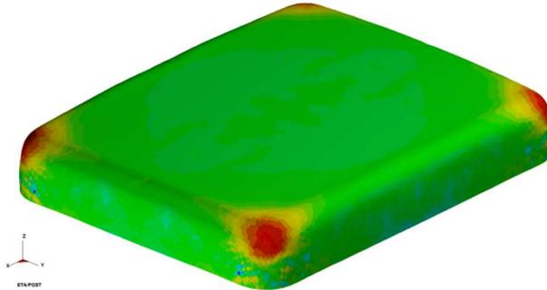
**Fig 8:** Thickness distribution of the finished product resulted after removing the technological addendum
