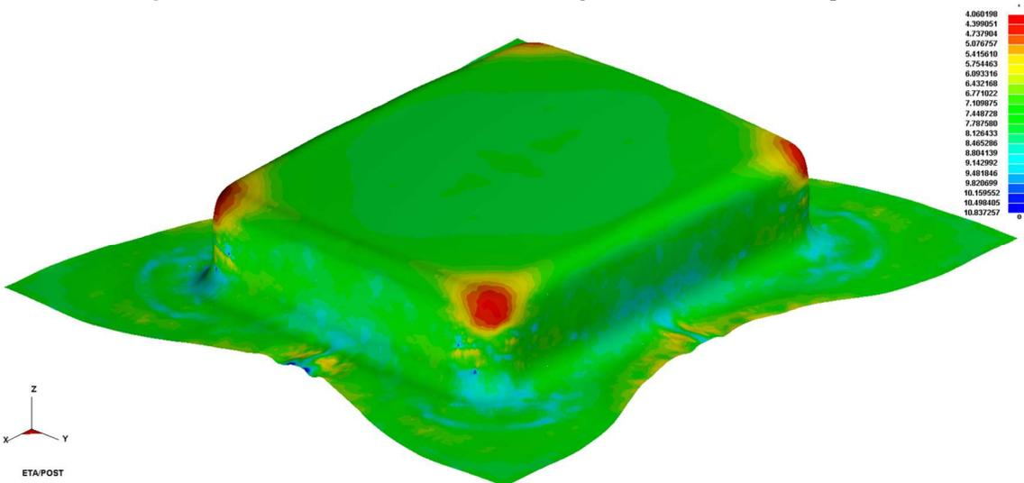
**Fig 6:** Thickness distribution at the end of the thermoforming process
