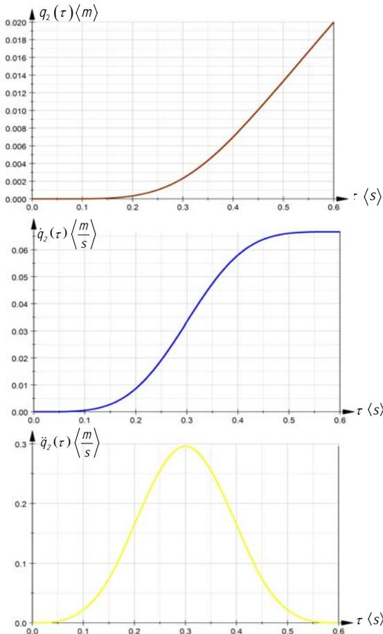
Fig.2 The time variation laws for coordinates, velocities and accelerations for 2TR robot
