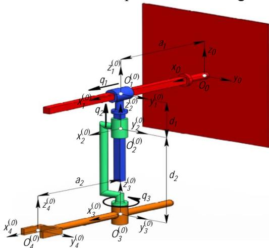
**Fig.1** The kinematical structure of 2TR robot
