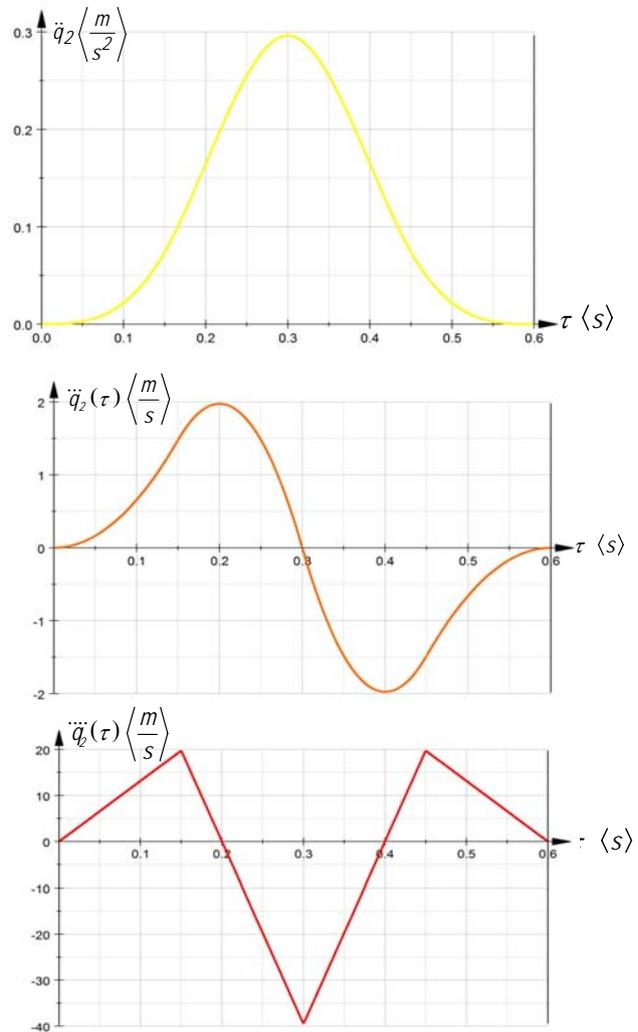
Fig.3 The time variation laws for accelerations of first, second and third order for 2TR robot
