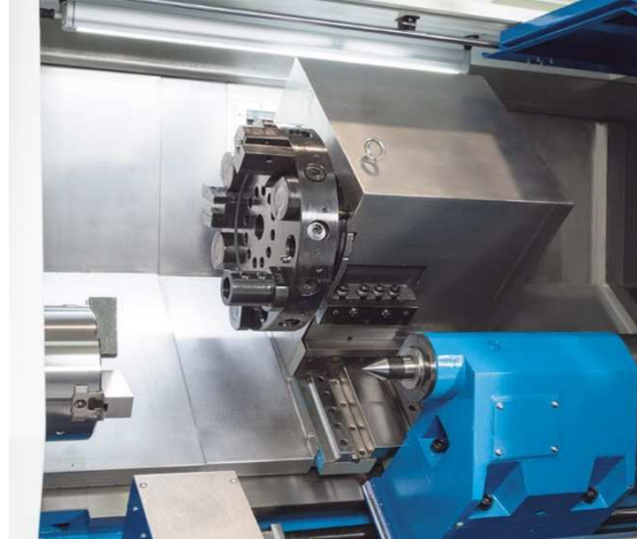
Fig. 1: Turning machine with inclined bed frame
