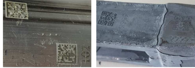
Fig.7: QR-Codes generated by fibre-laser: Aluminium at 550°C damaged by collisions (left); Steel at RT covered by an oxide-layer development at 900°C for three hours (right). All codes have been recognised successfully.
