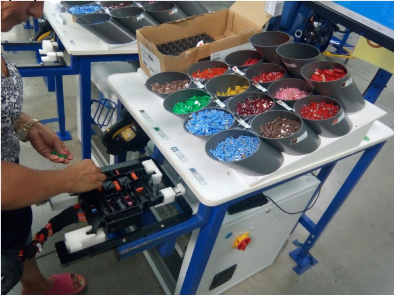
Fig. 2: The current state of fuse mounting within the enterprise
