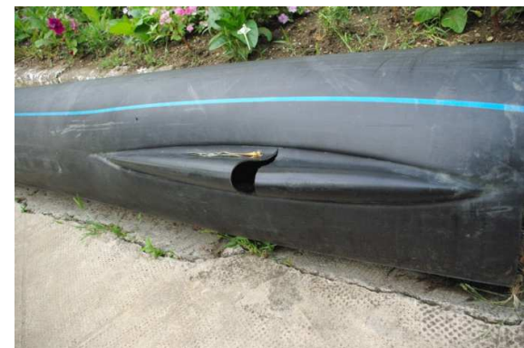
Fig. 13. The rupture "parrot beak"
