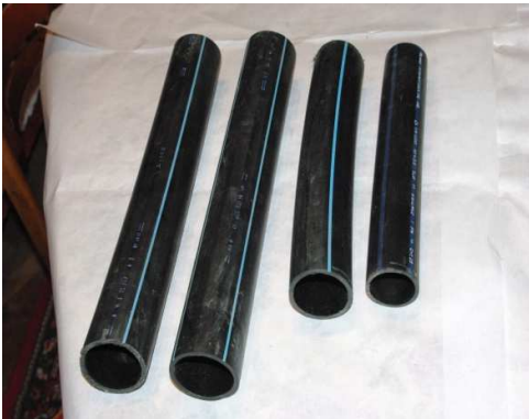
Fig.3. Types of polyethylene pipes used in distribution network
