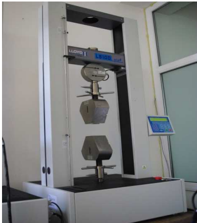
Fig.14. Testing machine tip Lloyd LS 100 and a tube \Phi 20 \times 2
