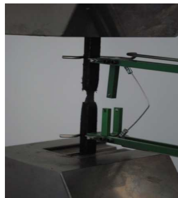
Fig. 16. The extensometer used
