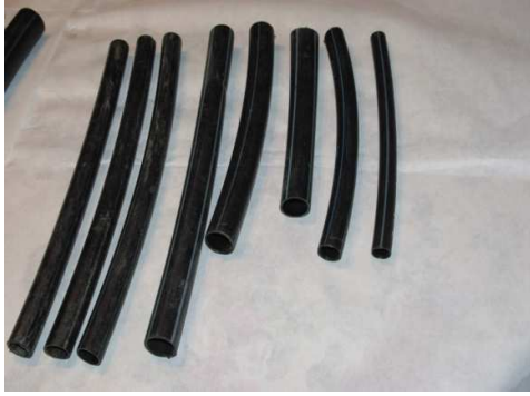
Fig.2. Types of polyethylene pipes used in branch lines
