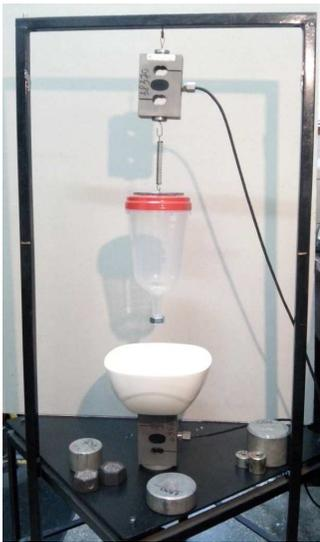
**Fig. 1.** General view of the experimental setup of the variable mass system
