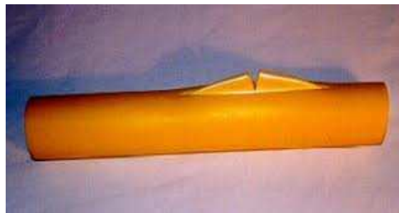
Fig.2. The "parrot beak" crack [37], [38]
