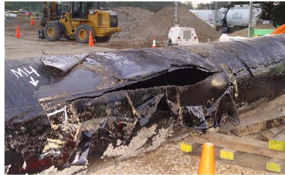
Fig.1. Ductile crack in a pressured tube [36]
