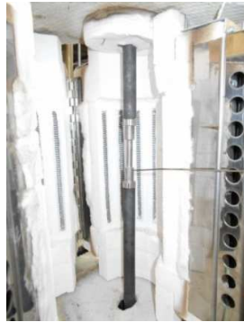
Fig. 2 Hot tensile testing apparatus and the sample.
