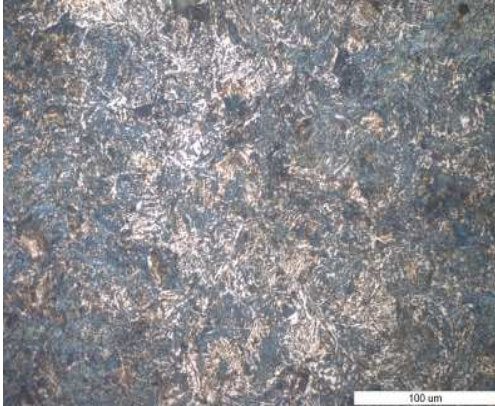
Fig. 1 Optical micrograph of as-received 42CrMo4 steel.
