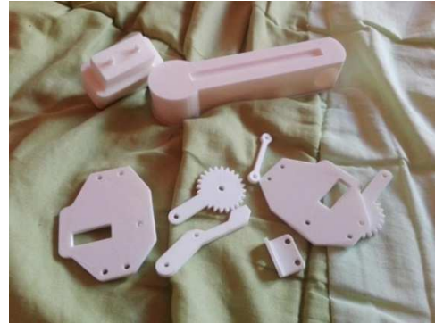
Fig. 12 Components obtained after 3D printing After all the parts for the robotic arm have been created (figure 12), the next step was to assemble the robotic arm.
