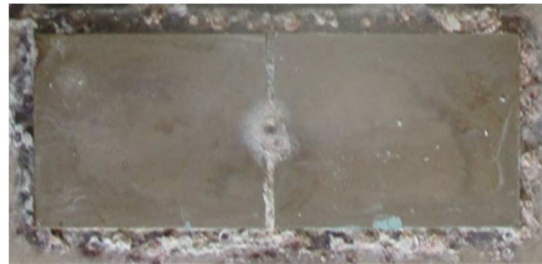
Fig. 2 Brazed joint after 600 hours of salt spraying.
