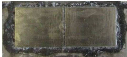
Fig. 4 Brazed joint after 600 hours of acetic acid spraying.
