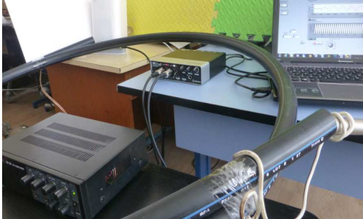
Fig. 4. Set-up with two channels USB sound card and sound amplifier
