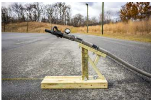
Fig.3. Water discharge by holding the discharge hose in a fixed position
