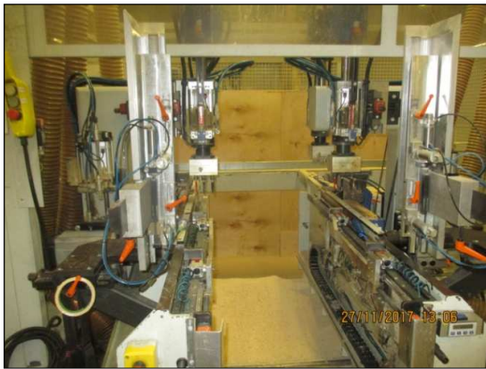
Fig. 2. The multiple drilling machine used for processing
