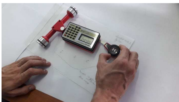
Fig. 1 The measurement of a productive area with digital planimeter
