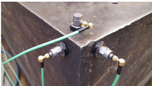
Fig. 6. The placement of the accelerometers
