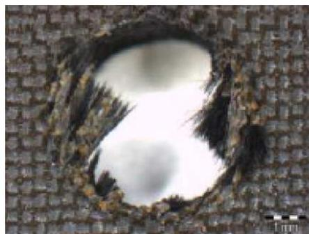
Fig. 1. Hole with delamination
