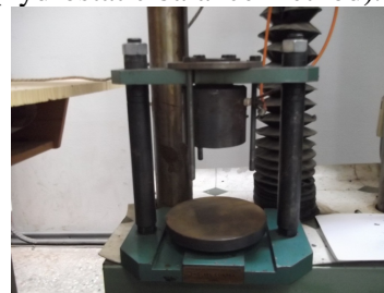
Fig.1. Experimental stand for injection molding - the injection device [UTCN].
