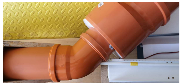
Fig. 3. Long tube A (left), elbow, large tube B (speaker inside), thin tube for microphone
