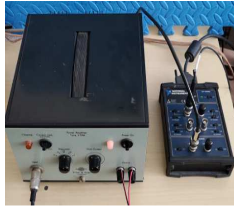
Fig. 2. Signal conditioning unit (right) and the power amplifier
