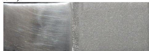
Fig. 2. The beam produced with SLM technology (two surfaces prepared: mirror texture and sandblasted with aluminium oxides 120µ granulation, at 4 atm. pressure).
