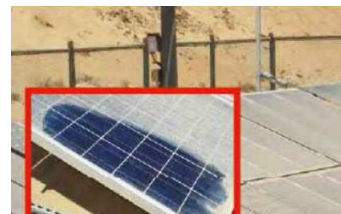
Fig. 1. P-V arrays covered by dust in desert area [8].
