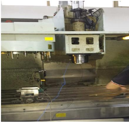
Fig. 3. Positions of sensors.
