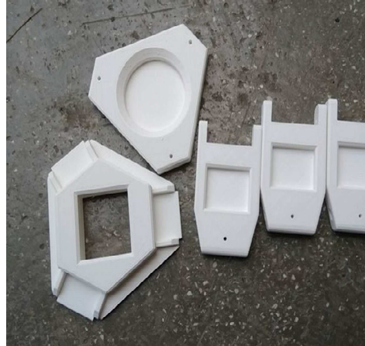
Fig. 7 Main components of the Delta robotic system
