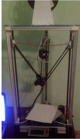
Fig. 10. The prototype of the Delta printer
