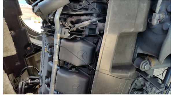
Fig. 9. Vibrometer site for vibration measurement at point P6
