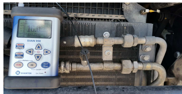
Fig. 7. Accelerometer position for the 4 point
