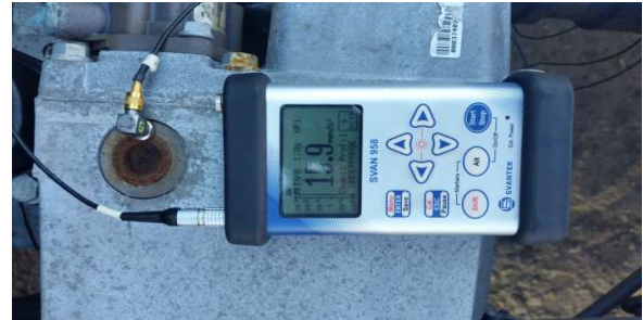
Fig. 3. Vibrometer in the point P1 on the truck motor
