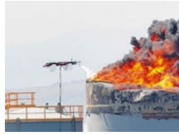
Fig. 6 Water jet equipped drone [4]
