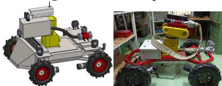
Fig. 12 ROV for firefighting – CAD model and mocup
