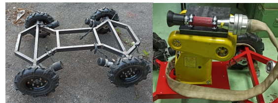
Fig. 21 Mockup: a) chasy with motors and wheels, b) discharge nozzle on the robotic arm
