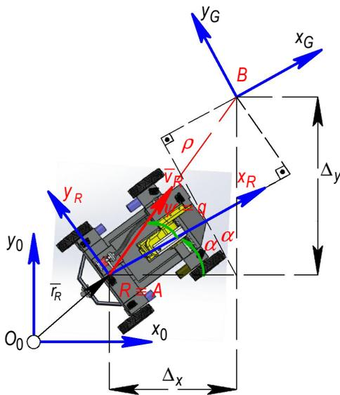
**Fig.4** The parameters of the mobile robot in polar coordinate system
