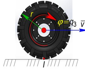
Fig.3 The velocities of the wheels
