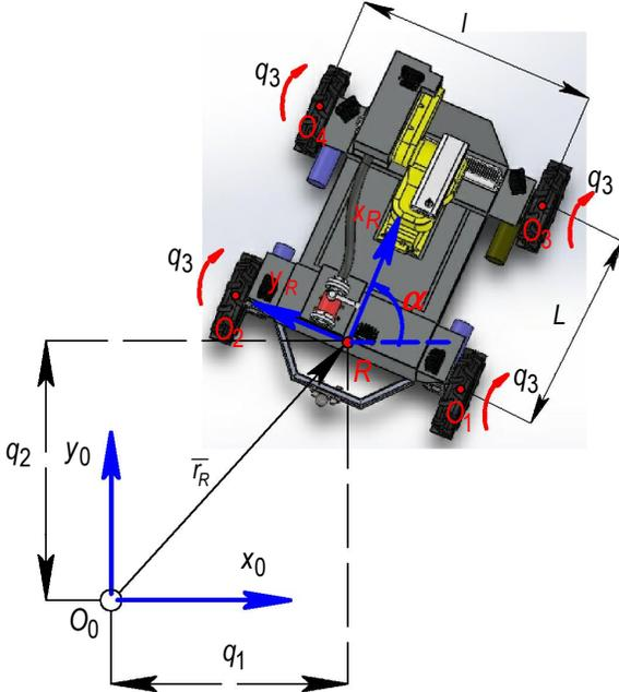
Fig.2 The independent parameters of the mobile robot
