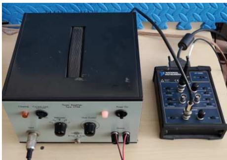
Fig. 4. The NI signal conditioning unit and the power amplifier
