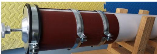
Fig. 2. Screw for the rigid termination displacement and the air layer thickness setting
