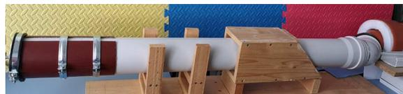
Fig. 1. The simple impedance tube - overview
