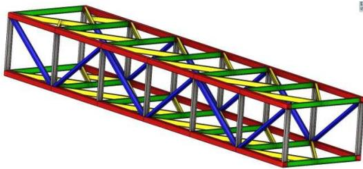
Fig.3. The middle section of the BWE boom
