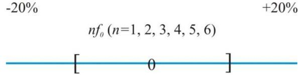
Fig.12 The safety limits of the resonance frequencies
