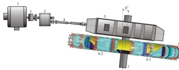
Fig.5 The parts of the drive mechanism of the bucket wheel
