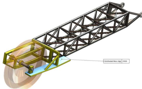
Fig.6 Model of the drive mechanism using a uniform distributed mass
