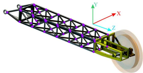
Fig.9 The nodal network of the beam structure and the coordinate system
