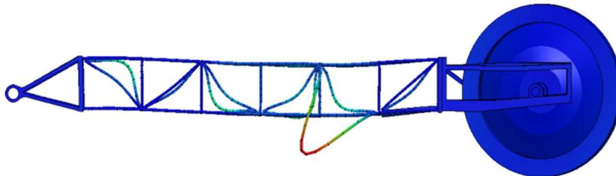
Fig. 21 Deformation of the boom on direction Z for mode 10 (16.84 Hz - in the presence of the boom's hoisting cables and considering gravity)
