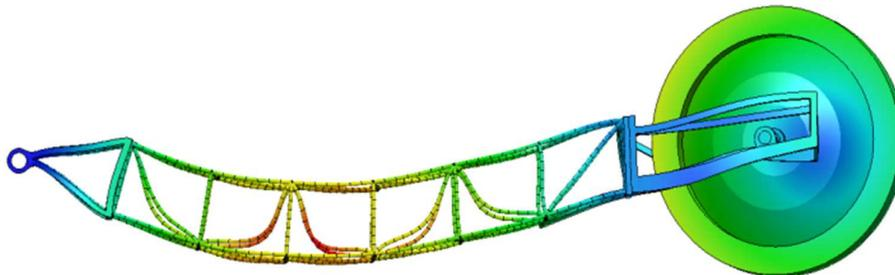
Fig. 20 Deformation of the boom on direction Z for mode 6 (9.2999 Hz - in the presence of the boom's hoisting cables and considering gravity)
