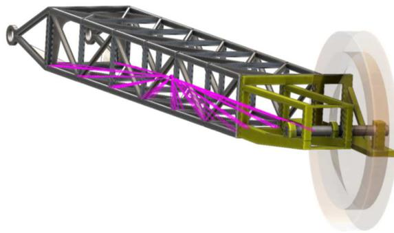
Fig.7 Model of the conveyor installed on the boom as a remote mass
