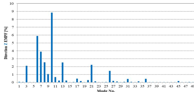
Fig.17 The EMPF for direction Z (in the presence of the boom's hoisting cables and considering gravity)
