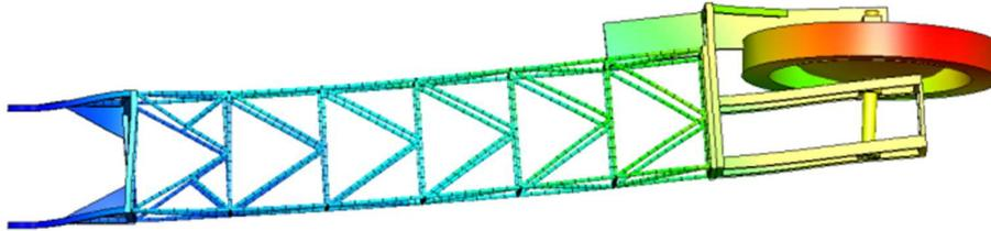
Fig.18 Deformation of the boom on direction X for mode 1 (1.9779 Hz - in the presence of the boom's hoisting cables and considering gravity)
