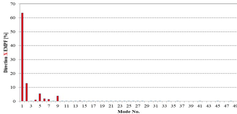
Fig.15 The EMPF for direction X (in the presence of the boom's hoisting cables and considering gravity)
