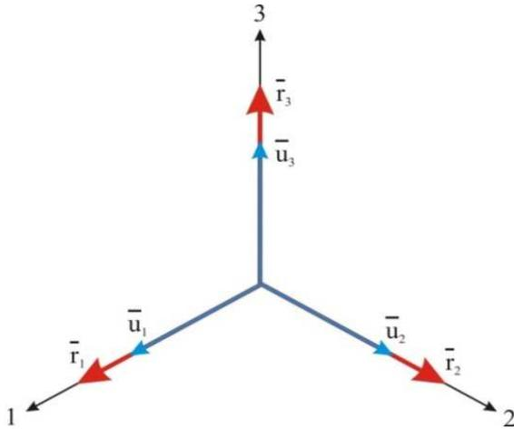
Fig.10 A rigid body's degrees-of-freedom (DoF) in the local coordinates system
