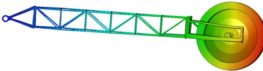
Fig. 19 Deformation of the boom on direction Y for mode 2 (2.1092 Hz - in the presence of the boom's hoisting cables and considering gravity)
