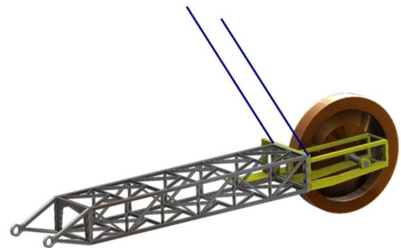
Fig.8 Model of the boom hoisting cables using two springs
