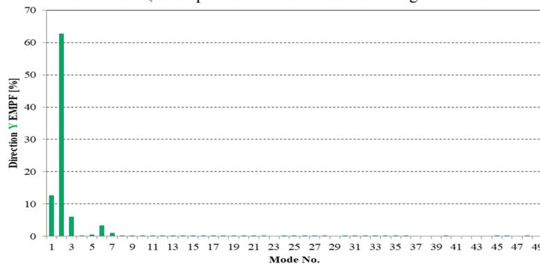
Fig.16 The EMPF for direction Y (in the presence of the boom's hoisting cables and considering gravity)
