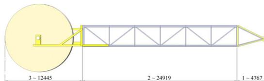
Fig.2 The parts of the model of the BWE boom
