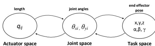
Fig. 1. Kinematic mapping between robot spaces
