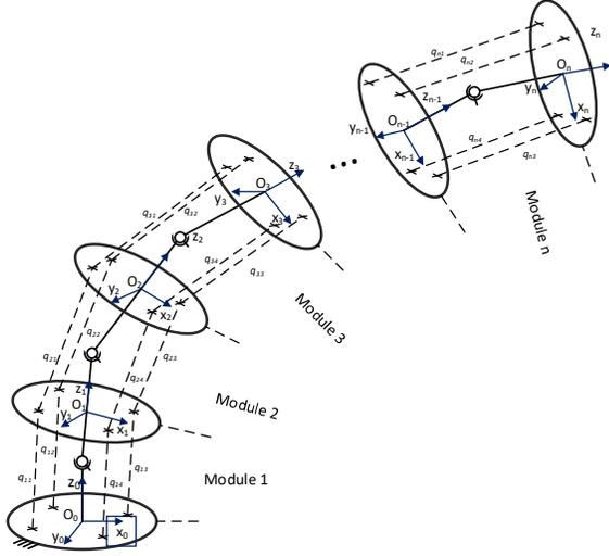
Fig. 2. The hyper redundant robot schematic representation
