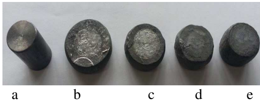
Fig.7 Deformed cylindrical samples on laboratory sonnet at different impact energies (unlubricated) a) initial sample; b) 48000 daN mm; c) 32000 daN mm; d) 24000 daN mm; e) 16000 daN mm
