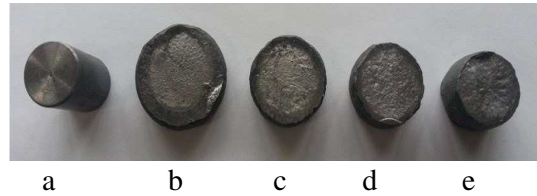
Fig.9 Deformed cylindrical samples on laboratory sonnet at different impact energies (lubricated with mineral oil) a) initial sample; b) 48000 daN mm; c) 32000 daN mm; d) 24000 daN mm; e) 16000 daN mm.
