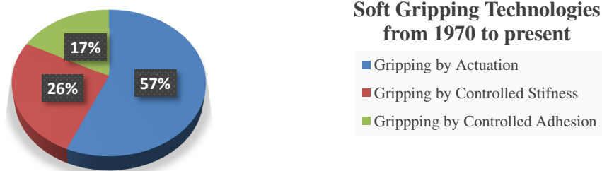
Fig. 2. Statistics of soft gripping technologies from 1970 to present.
