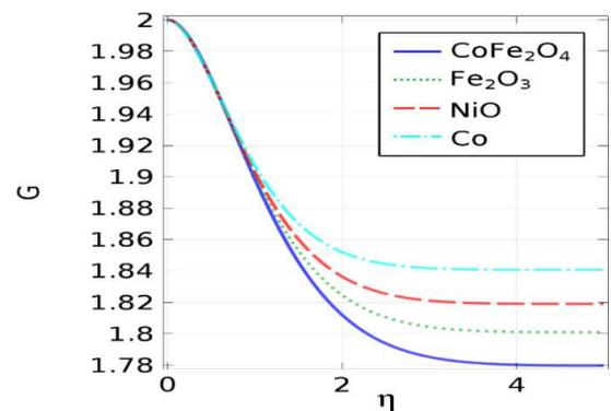
Figure 13: Axial velocity distribution for different nanofluids.
