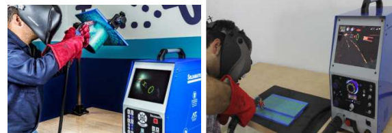
Fig. 12a. Welding position using SOLDAMATIC simulator.
