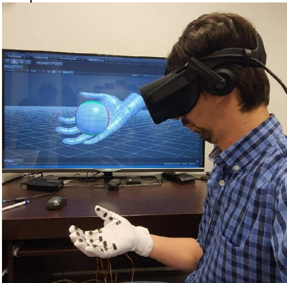
Fig. 12 Subject testing the interaction between haptic glove, HMD and the Virtual Reality environment
