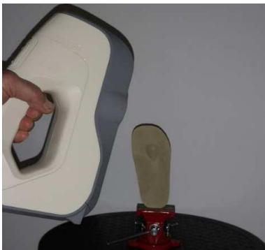
Fig.5. Scan method using ARTEC Eva Scan
