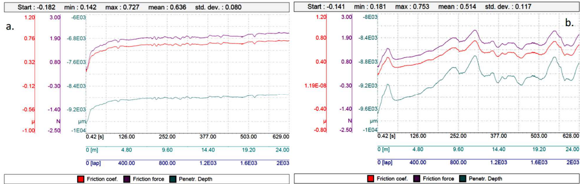
Fig.12. Tribological dependents for the samples based on Ti powders obtained by CS (a) and TSS (b)
