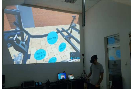
Fig. 14. Custom buttons positioned within the virtual reality training environment
