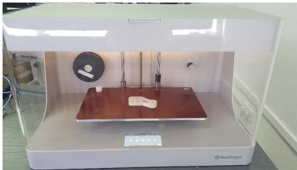
Fig. 4. Markforged MarkTwo 3D printer from TUCN.
