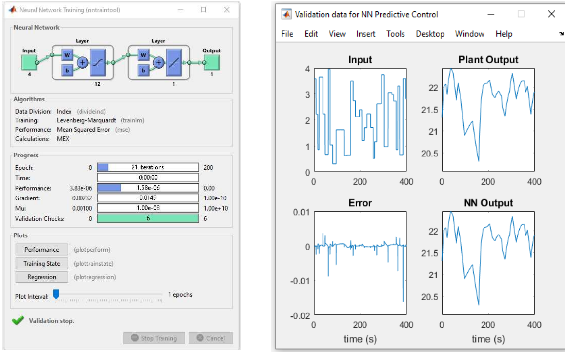
Fig. 9. Simulink model for neural control and graphical result of odor pump operation
