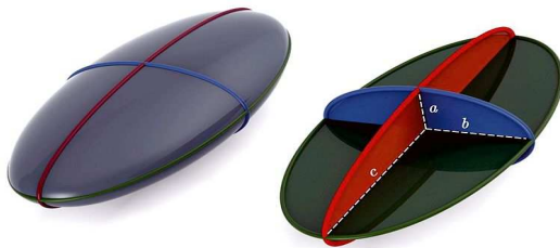
Fig. 2. Body ellipsoidal segment adapted to the left deltoid, with semiaxes: b – on the body direction x; c – on the body direction y; a – on the body direction z,
