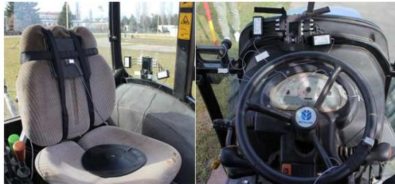
Fig. 3. Mounting the tri axial accelerometers on the tractor seat surface, on the seat back, respectively on the cab floor at the support leg
