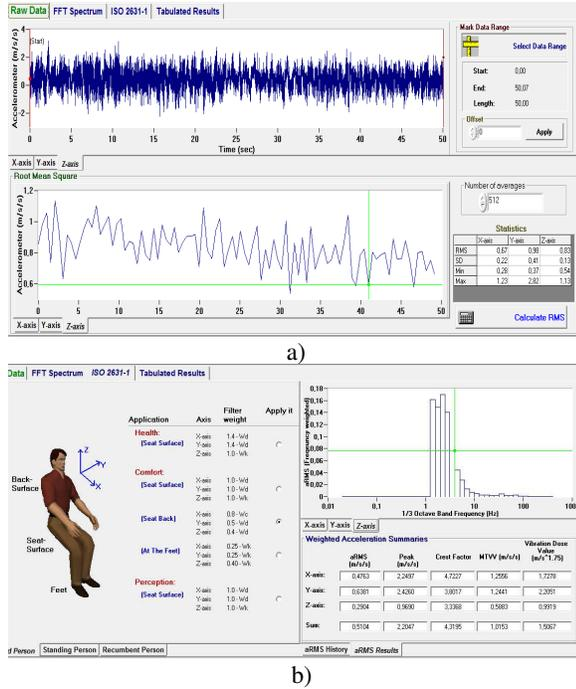
**Fig. 6.** a) Row data collected by ACL 2 (seat back) and b) the graph of aRMS, on Z axis for comfort zone; for arable land and tractor speed of 5 km/h.
