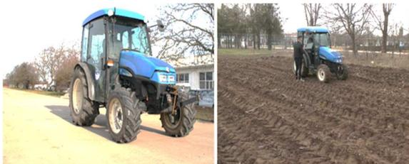
**Fig. 1.** Carrying out experimental tests on straight terrain and arable ground, according to the experimental protocol, at speeds of 5 and 10 km / h
