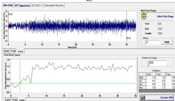
b) Fig. 4. Raw data and aRMS collected on straight road by the ACL mounted on the floor surface at the feet level; a) speed 5 km / h; b) speed 10 km / h
