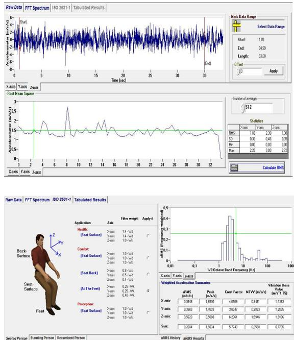
**Fig. 7.** Row data collected by ACL 3 (feet) and b) the graph of aRMS, on Z axis for comfort zone for arable land and tractor speed of 5 km/h.
