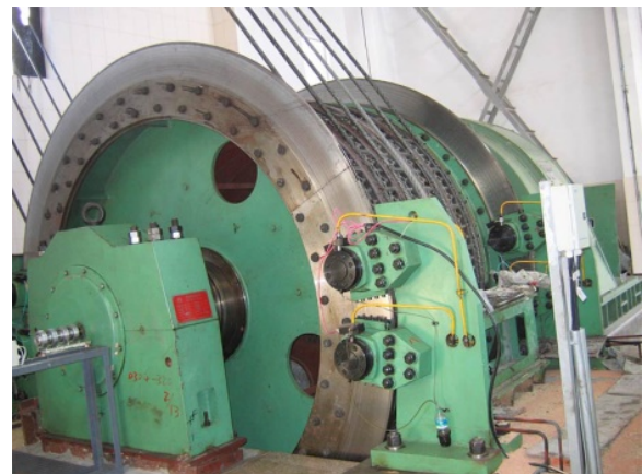
Fig.2. Mine hoist with disc and pad brake system
