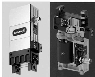
Fig. 1. SCHUNK-0310940 EGP 40NNB gripper 1- technological base of placement/fixing; 2- transversal guide system with rolls; 3- rack and pinion gear; 4- servomotor; 5- controller
