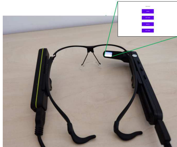
Fig. 9. One application page projected on Vuzix smart glasses
